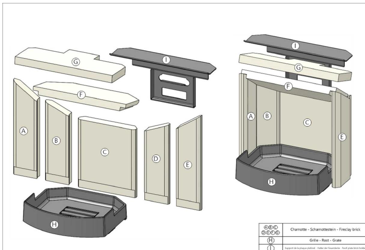
Chambre de combustion 2 | Brennkammer 2 | Burning chamber 2
