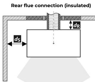
**Passage of the flue pipe through a wall made of combustible material**
