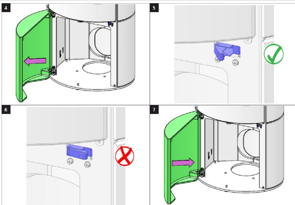
Chambre de combustion 1 | Brennkammer 1 | Burning chamber 1
