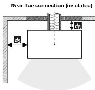
**Passage of the flue pipe through a wall made of combustible material**
