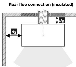
**Passage of the flue pipe through a wall made of combustible material**
