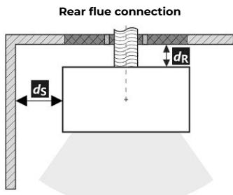
**Passage of the flue pipe through a wall made of combustible material**
